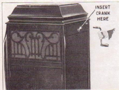
Fig. 6—The winding crank fits into the escutcheon or winding shield on all Cecilian models. This crank winds the main spring which is made of finely tempered steel and furnishes power to the motor.
