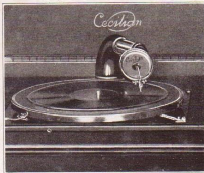
Fig. 12.—Here is how the reproducer appears properly turned over, and in a position to play an Edison or old style Pathe record. Note that a different type of needle is required for these records.
