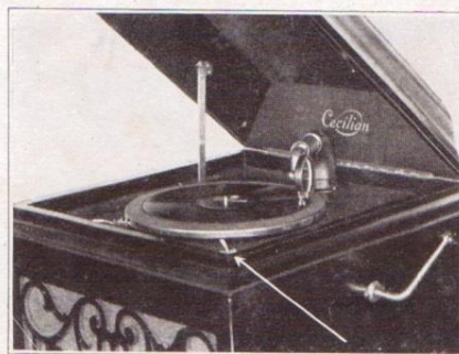
Fig. 15—The arrow indicates the speed regulating dial on the motor board. If you use your Cecilian four or five times a week the speed regulator will need to be adjusted to keep the music pitch at the right tone.
