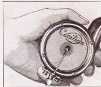
Fig. 11—To play an Edison record, grasp the reproducer and turn it clear over to the left, so that the diaphragm is at a right angle to the tone arm.
