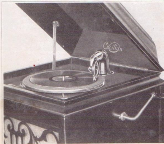
Fig. 9—The tone arm is not swung into place at the right edge of the record until the motor is running at full speed. Do not touch or jar the face of the reproducer, as the delicate sound amplifier may become injured.
