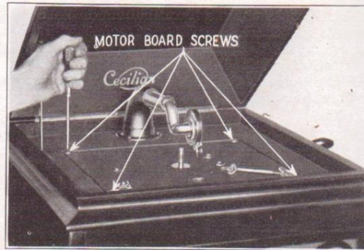
Fig. 16—Lift the turn table off the spindle so that you can unfasten the motor board screws in each corner of the board. They can be removed with a screw driver.
